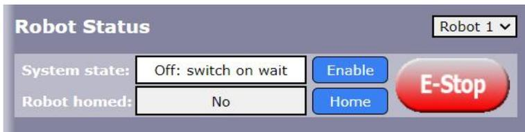
Figure 4-3: Robot Status Section of the Virtual Pendant
